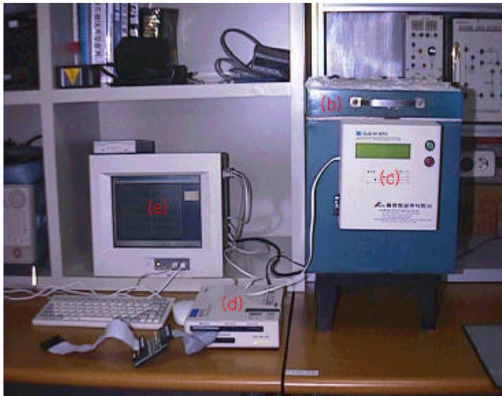
Fig. 4.1 Electric furnace controller for heat treatment using Internet
