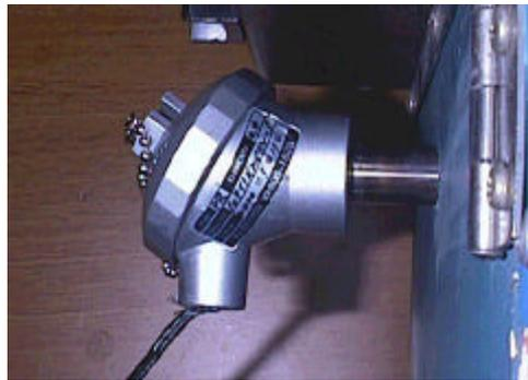
Fig. 4.6 "R" type temperature sensor
