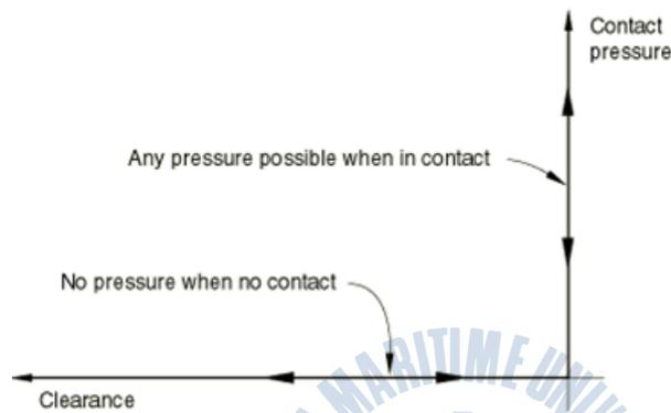
Fig. 3-10 Default pressure-overclosure relationship of “hard”contact
