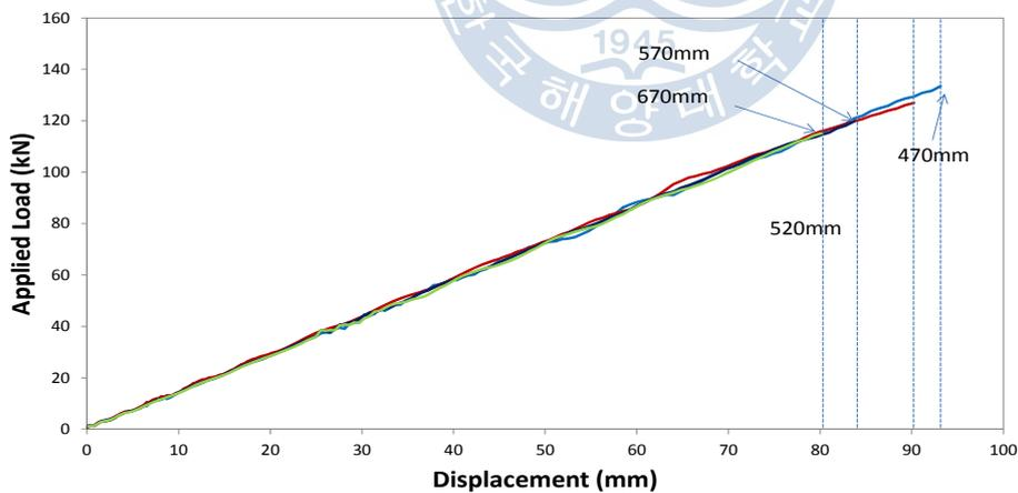
Fig. 4-33 Parametric study on width of spiral rebar
