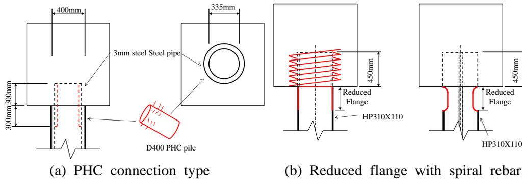
(a) PHC connection type (b) Reduced flange with spiral rebar connection
