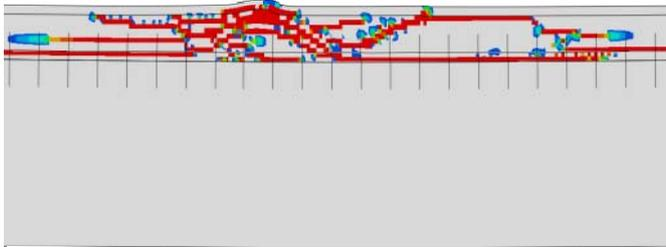
(b) Crack patterns in mid-span
