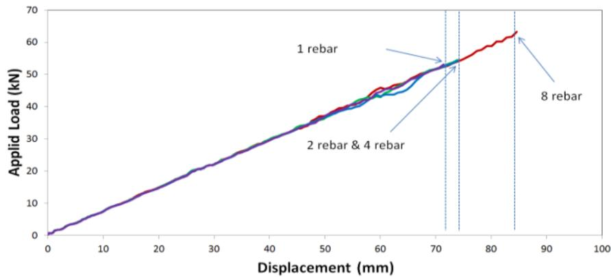
Fig. 4-35 Parametric study on quantity of square rebar
