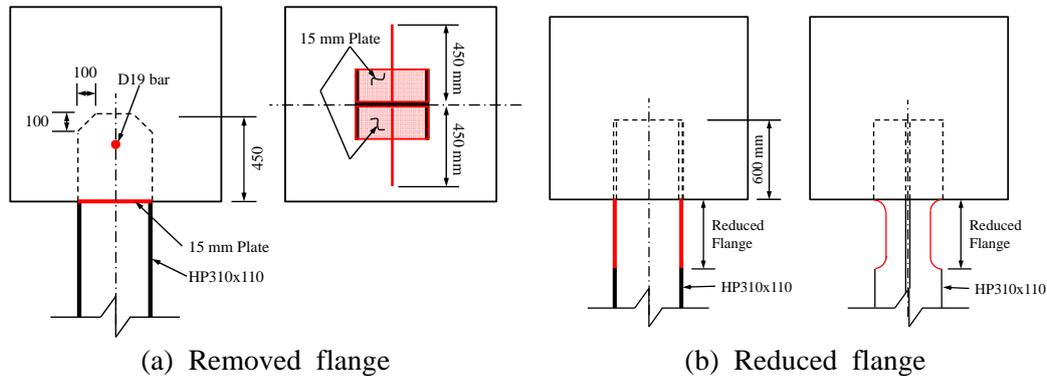
Fig. 4-12 Detail of removed flange and reduced flange connection type
