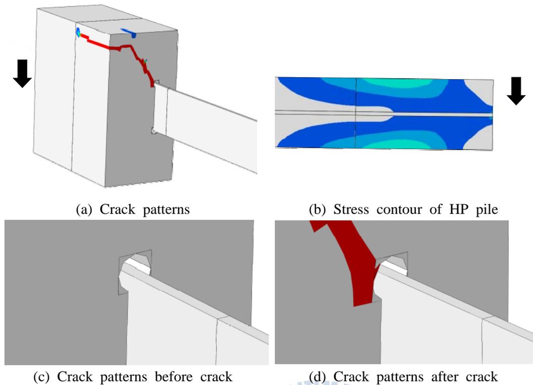
Fig. 4-23 Crack patterns and stress contour of hole connection type
