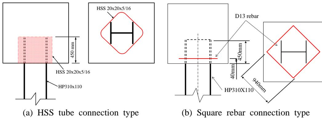
Fig. 4-10 Detail of HSS tube connection type and square rebar connection type
