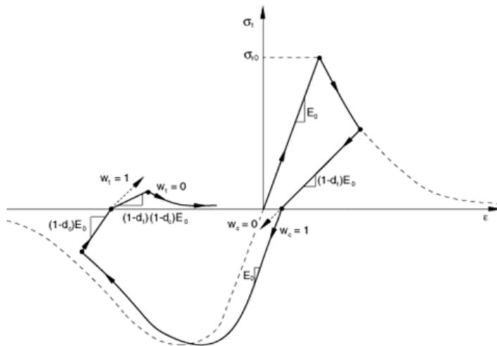
Fig. 3-5 Uniaxial load cycle curve (tension-compression-tension)
