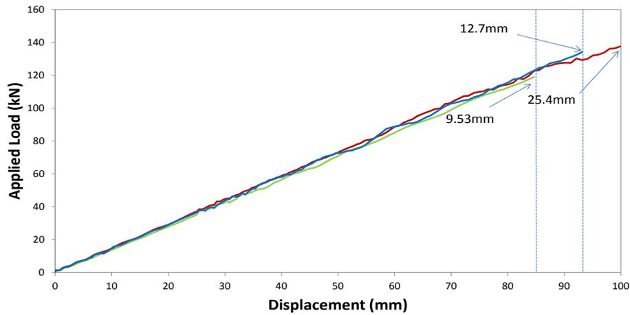
Fig. 3-32 Parametric study on diameter of spiral rebar
