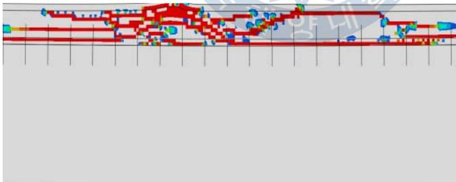
(b) Crack patterns in mid-span
