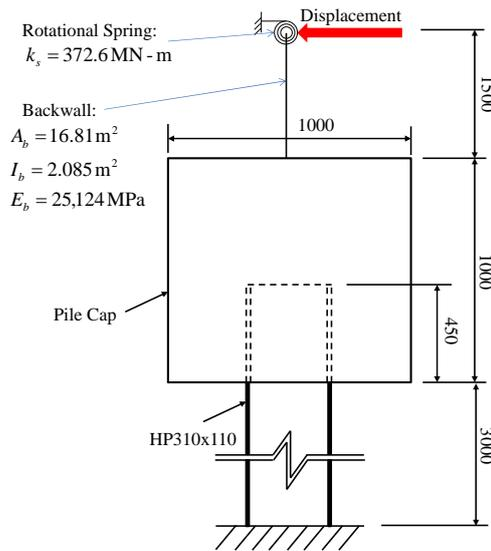
Fig 4-1 Schematic of numerical model setup
