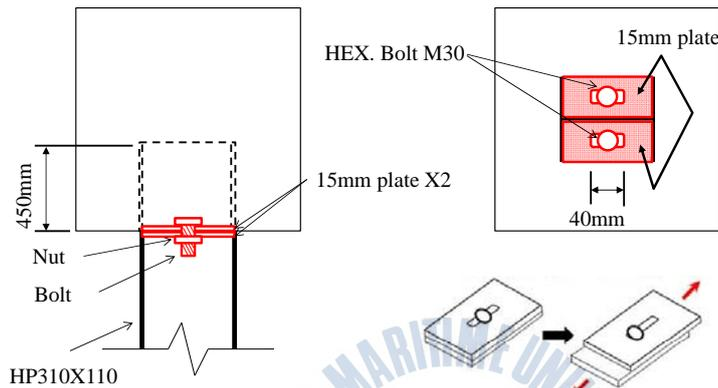
Fig. 4-15 Detail of slot connection type
