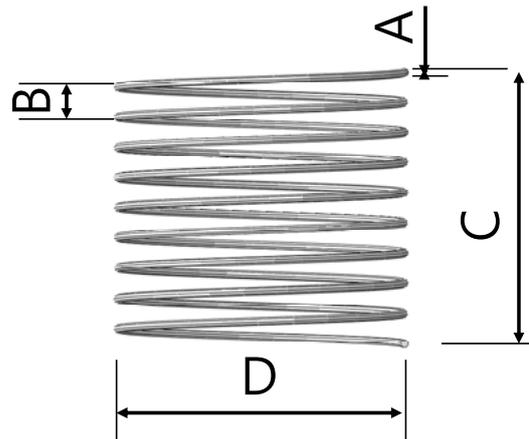
Fig. 4-30 Parameter of spiral rebar
