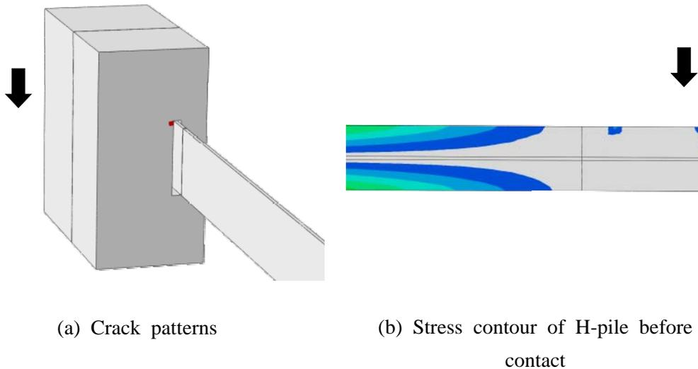
(a) Crack patterns (b) Stress contour of H-pile before contact
