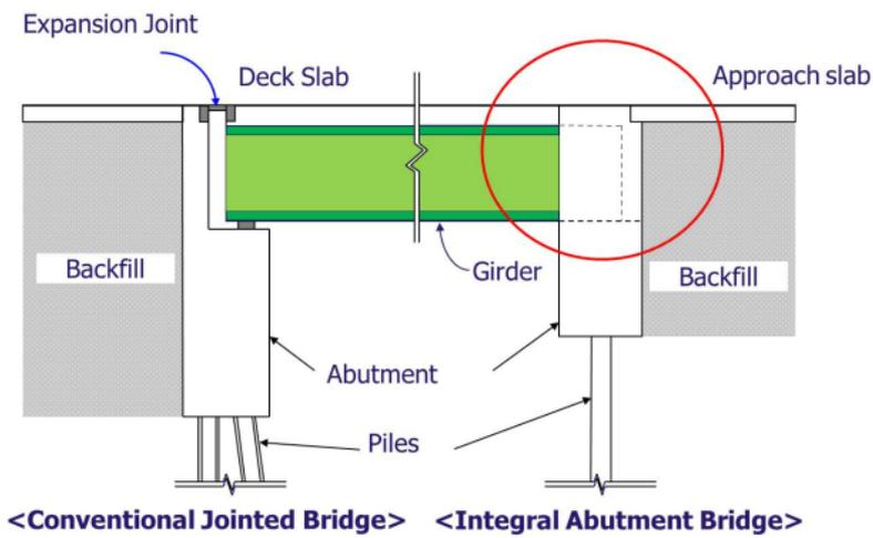
Fig. 1-1 Schematic of conventional jointed bridge and integral abutment bridge (Kim et al., 2013)
