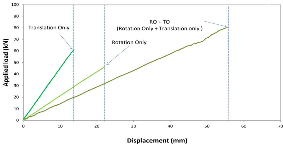
Fig. 4-8 Load-displacement graph depending on boundary conditions
