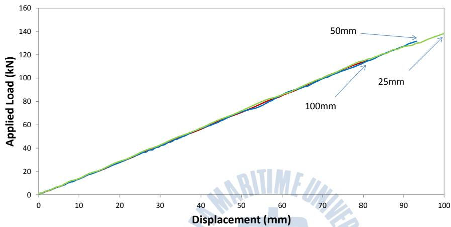
Fig. 4-31 Parametric study on pitch spacing of spiral rebar
