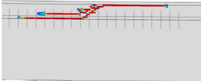
(b) Crack patterns in mid-span
