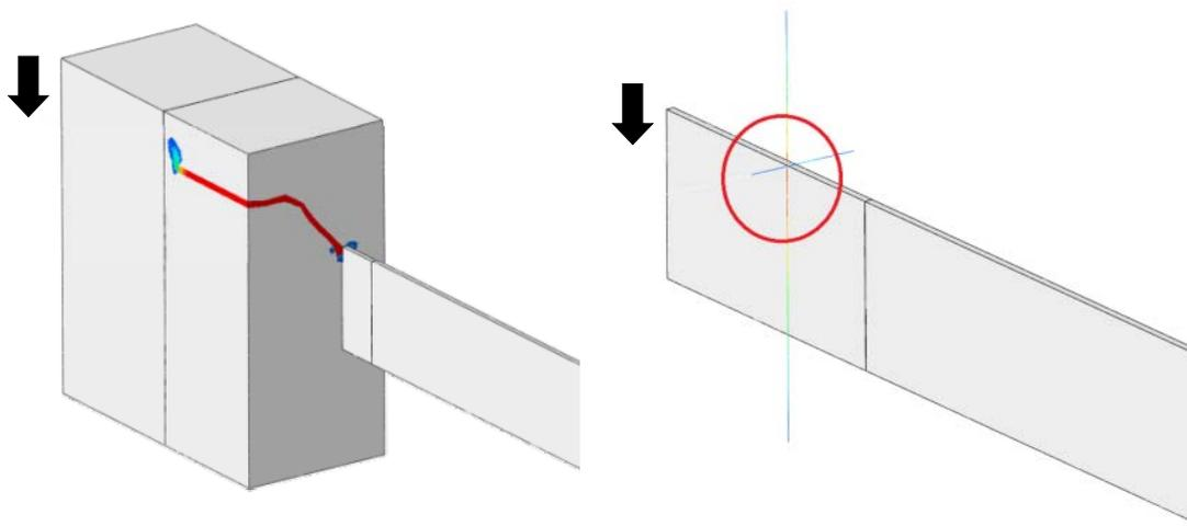
(a) Crack patterns (b) Plastic strain
