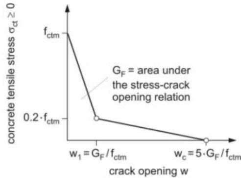
Fig. 3-4 Stress-crack opening relation for uniaxial tension
