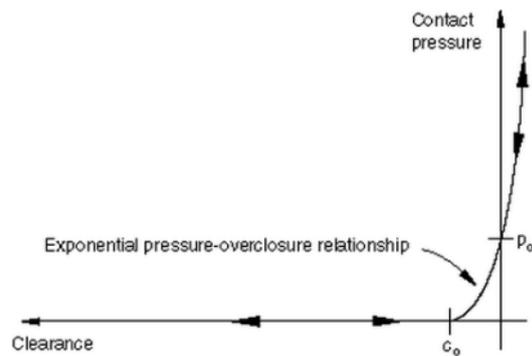
Fig. 3-9 Exponential “softened” pressure-overclosure relationship in Abaqus/Explicit
