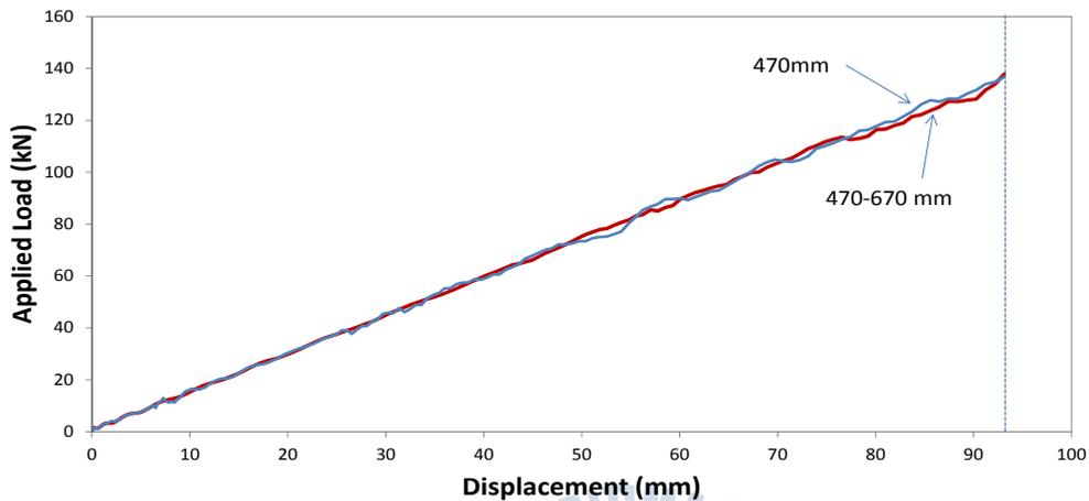
Fig. 4-34 Results of asymmetry spiral rebar
