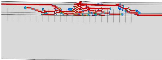
(b) Crack patterns in mid-span
