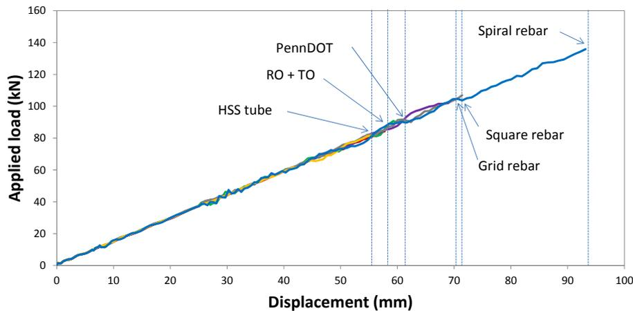
Fig. 4-28 Load-displacement curves obtained from increased stiffness connection types
