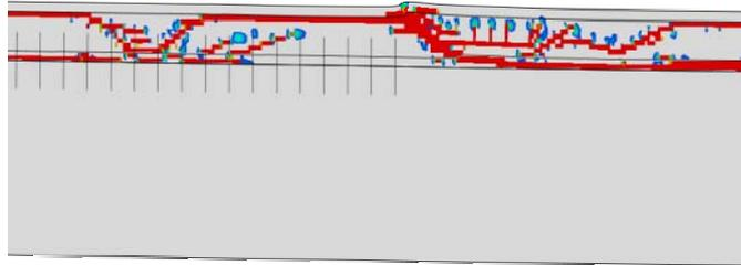
(b) Crack patterns in mid-span
