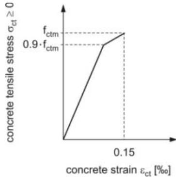
Fig. 3-3 Schematic representation of the stress-strain for uniaxial tension
