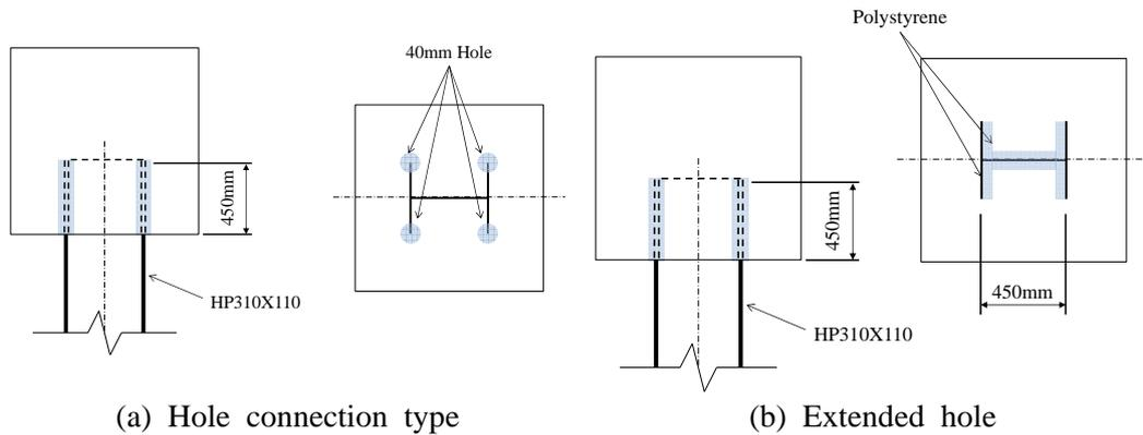
Fig. 4-13 Detail of hole connection type and extended hole connection type
