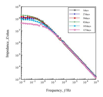
Fig. 12. Change of impedance characteristics with time for ZPC-pigmented film exposed to 0.5M-NaCl solution.(Alkyd resin)
