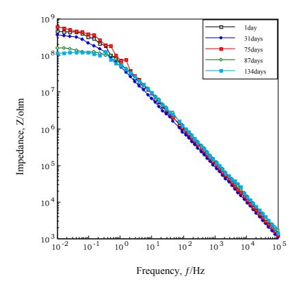
Fig. 19. Change of impedance characteristics with time for Fe<sub>2</sub>O<sub>3</sub>-pigmented film aged in Weather-Ometer.(Alkyd resin)
