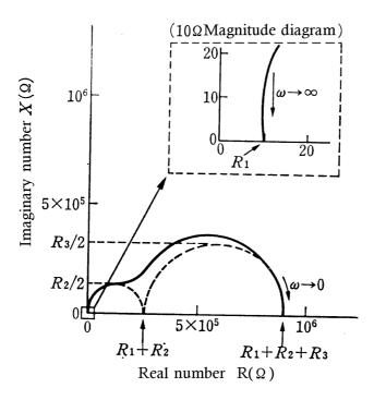
Fig. 3. Calculated impedance diagram(Nyquist plot) for degraded coated steel.
