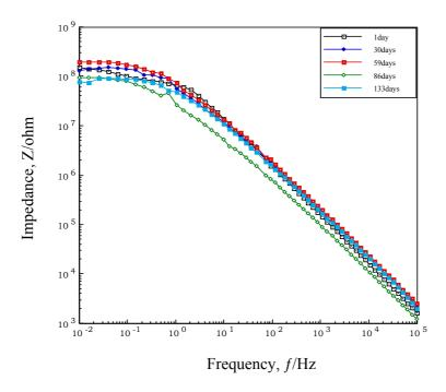
Fig. 18. Change of impedance characteristics with time for STC-pigmented film aged in Weather-O-meter. (Alkyd resin)
