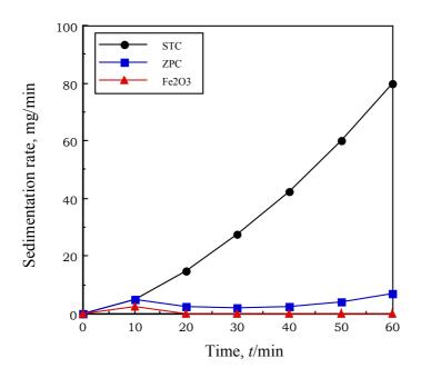
Fig. 8. Sedimentation rate of STC, ZPC and  $Fe_2O_3$  pigments in alkyd resin.
