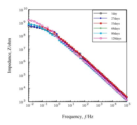
Fig. 22. Change of impedance characteristics with time for ZPC-pigmented film aged in Weather-O-meter. (Urethane resin)
