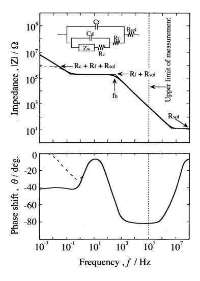
Fig. 4. Equivalent circuit and calculated impedance
