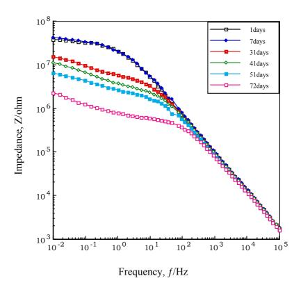
Fig. 13. Change of impedance characteristics with time for STC-pigmented film exposed to 0.5M-NaCl solution.(Urethane resin)
