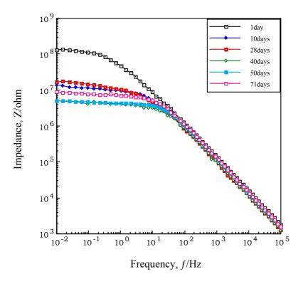
Fig. 11. Change of impedance characteristics with time for  $Fe_2O_3$ -pigmented film exposed to 0.5M-NaCl solution.(Alkyd resin)
