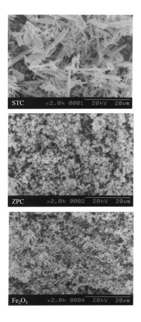
Fig. 7. Scanning electron microscopy of anti-corrosion pigments.
