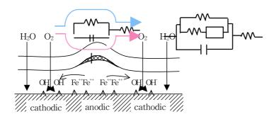
Formation of OH reaction with diffusing Fe<sup>++</sup> results in formation of rust of the cathodic areas of the steel surface
